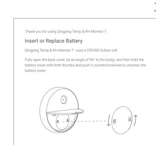
If the screen doesn't display anything, the battery needs to be replaced.
