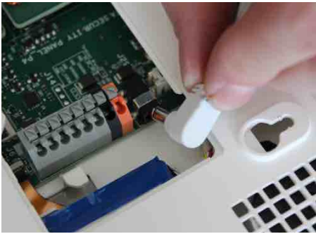
Plug in the power connector
