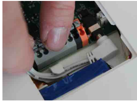
Route the wire behind the retainer clip
