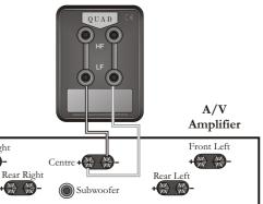
Choose a suitable length of twin core speaker cable, and prepare the ends as described.
