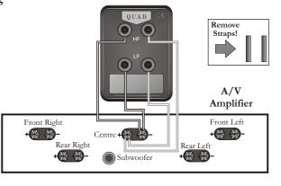
Most of the audio signal going to the speakers drives the bass units. Where one cable feeds both bass and treble units, this heavy bass current can modulate the high frequencies. Using separate cables for treble and bass units reduces intermodulation effects and improves headroom and clarity. This technique of wiring is known as Bi-Wiring. To bi-wire, you will need to install two lengths of twin core cable between the amplifier and each loudspeaker.
