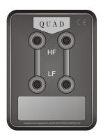
Quad crossovers separate the treble and bass networks into two distinct sections, each connected by a dedicated pair of terminal posts. This enables the treble and bass components to be separately driven for optimum performance. The upper pair of terminals is connected to the treble network and the lower pair to the bass network.
