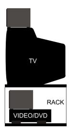
The loudspeaker should be positioned centrally between the loudspeakers close to the television and mounted either above or below the screen.
