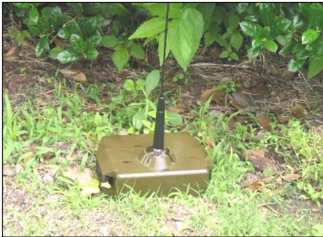
Operational Mode Flat and Level
