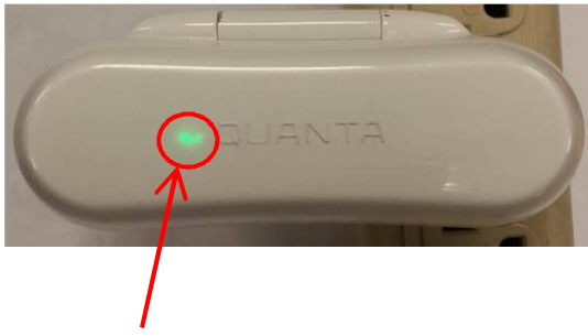
The green LED lights up after charging
