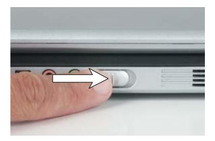
The power switch is preset to On/Off mode. However, you can also set it to function in Standby/Resume mode. For instructions on changing the power switch mode, see "Changing power settings" on page 178.
