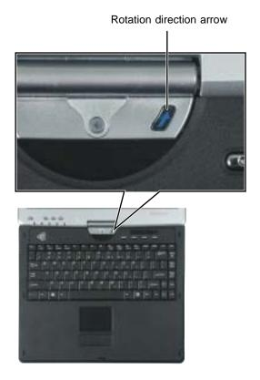
**3** Rotate the LCD panel in the direction of the rotation direction arrow until the panel is backwards.
