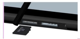
3. Carefully slide the microSD card into the microSd slot (as shown) until it "clicks" into place.
