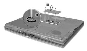
3 Insert the memory module diagonally into the slot (a), then gently press it down (b) until it clicks into place.
