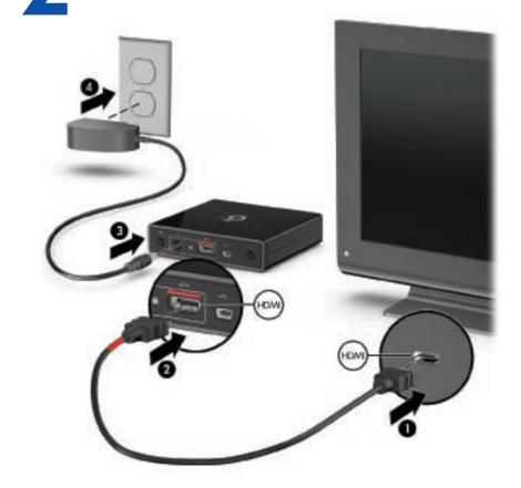
If you connected to a TV, press the input source button on the TV to select the HDMI input. When the components are connected correctly and the correct source is selected, the image on the computer display will be shown on the TV.
