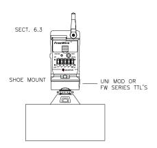
Connect the Hot Shoe Adapter FW12 or Uni-Mod FW11 to a Transmitter FW9T and slip it into a camera hot shoe.
