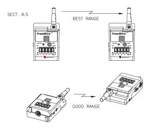
At close range (about 50' or 16m) antenna orientation is not critical. Antenna orientation matters more as distance between Transmitter FW9T and Receiver FW8R increases.
