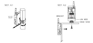
**5.2 Mounting directly to a bracket:** Use the #8/32 screw included with FreeWire to secure it through a hole in a bracket. Any other screw used must protrude not more than 3/4" (2 cm) into the FreeXwire case, or you will damage FreeXwire!
