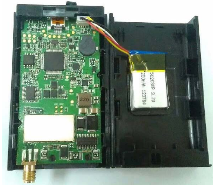
Figure 5. Backup Battery Installation
