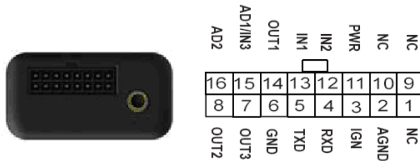
Figure 2. The 16 PIN connector on the GV300C
