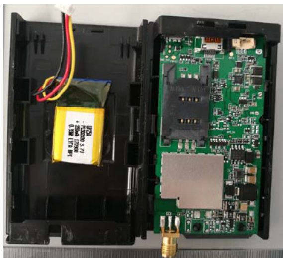
Figure 5. Backup Battery Installation
