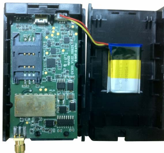
Figure 6. Backup Battery Installation
