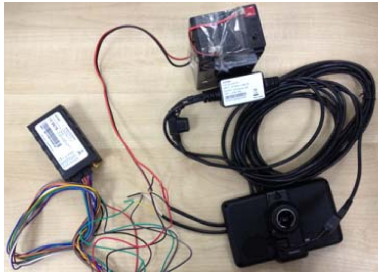
Figure 18. GV300 Connection with Garmin GPS Set
