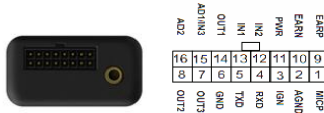
Figure 2. The 16 PIN Connector on the GV300N
