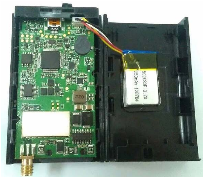
Figure 5. Backup Battery Installation
