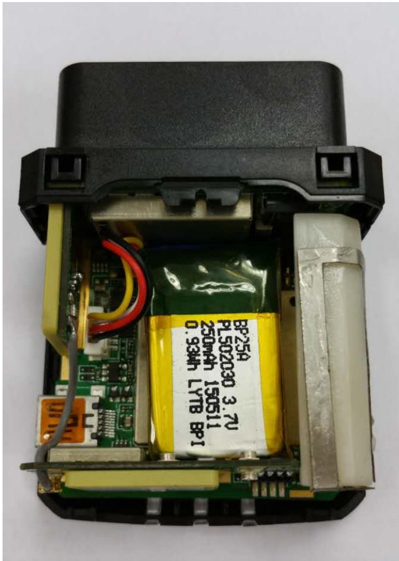
Figure 5. Backup Battery Installation
