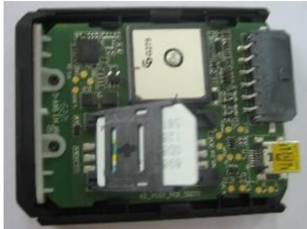
Figure 5. SIM Card Installation
