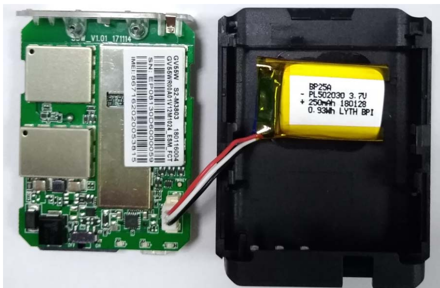
Figure 6. Backup Battery Installation
