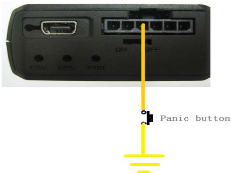
Figure 10. Typical Digital Input Connection
