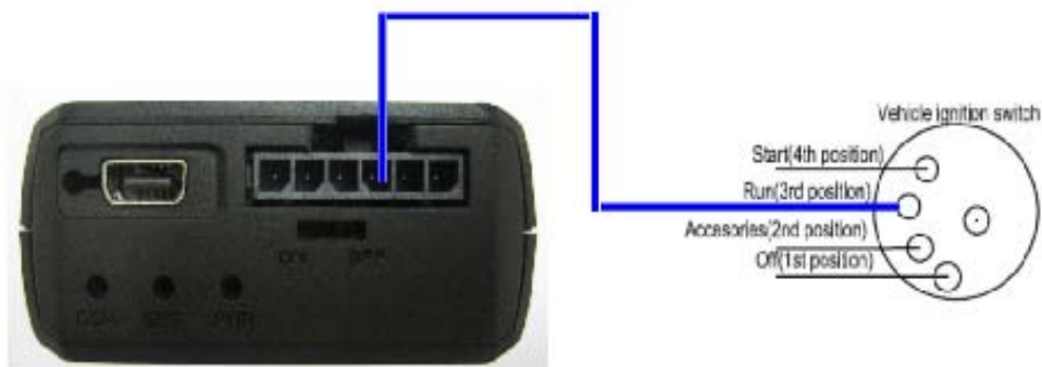
Figure 9. Typical Ignition Detection
