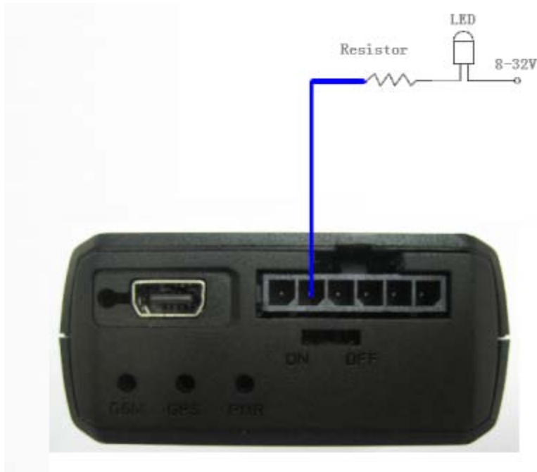
Figure 13. Typical Connection with LED
