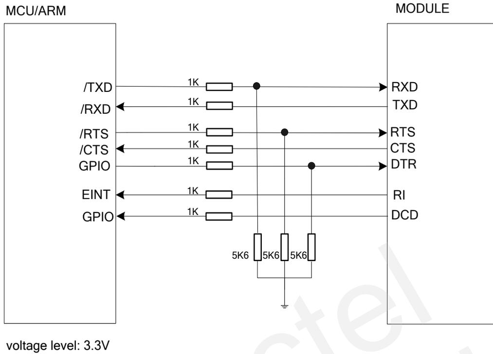
Figure 23: 3.3V level match circuit
