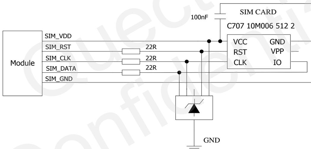
**Figure 30: Reference circuit of the 6 pins SIM card**
