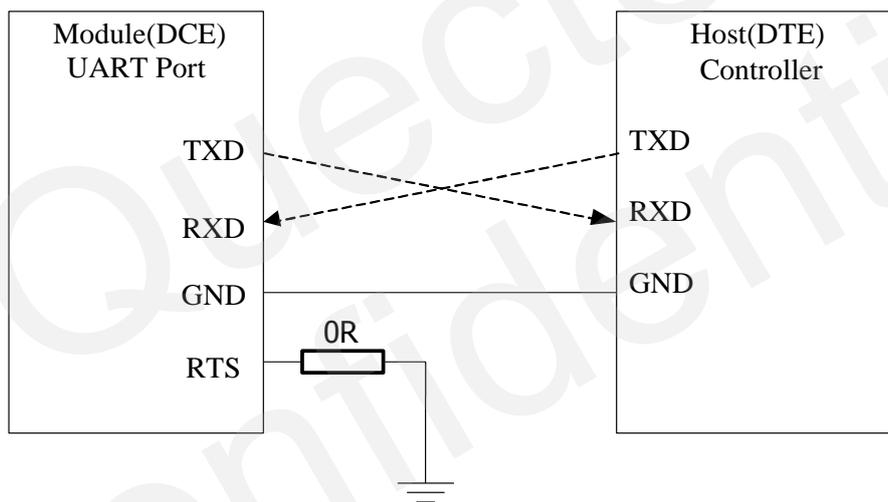
**Figure 19: Connection of three lines UART port**
