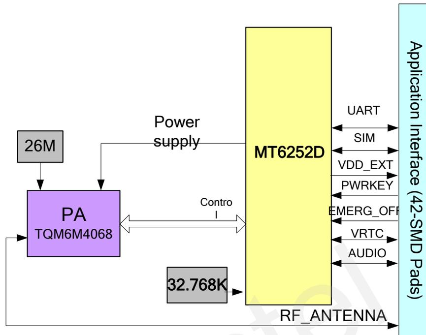
Figure 1: Module functional diagram
