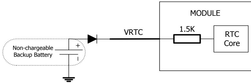
Figure 14: RTC supply from non-chargeable battery
