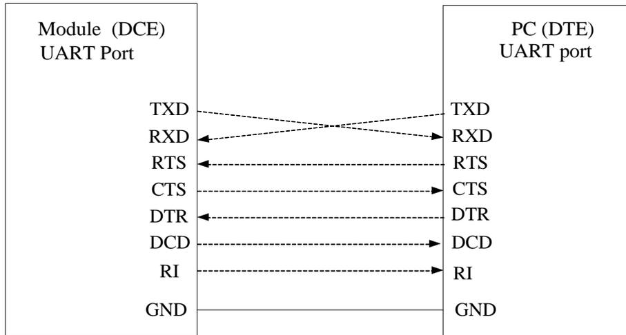
**Figure 18: Connection of all functional UART port**
