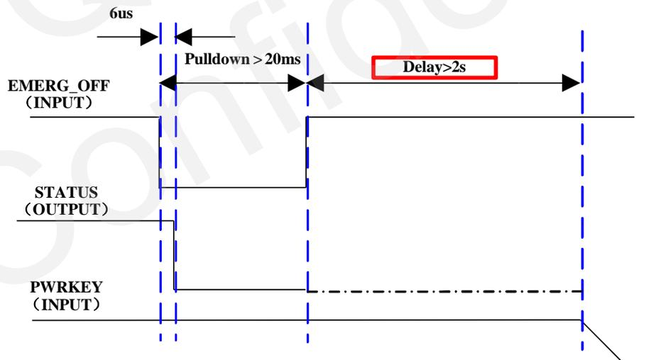
Figure 13: Timing of restarting system after emergency shutdown
