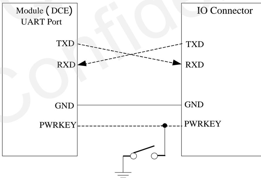
**Figure 21: Connection of software upgrade**
