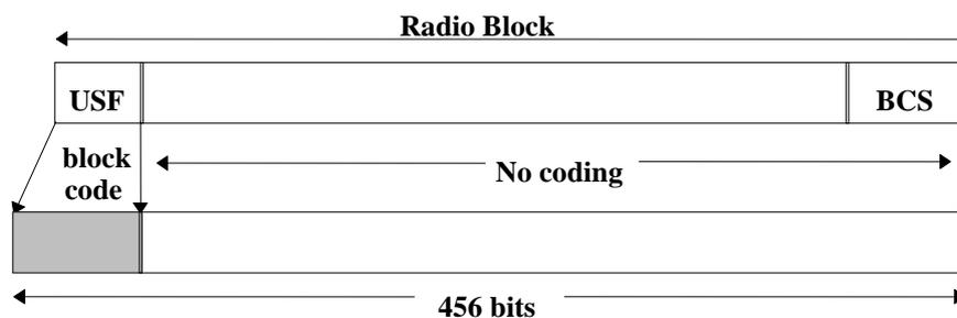
**Figure 49: Radio block structure of CS-4**
