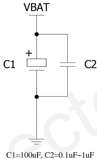
**Figure 4: Reference circuit of the VBAT input**
