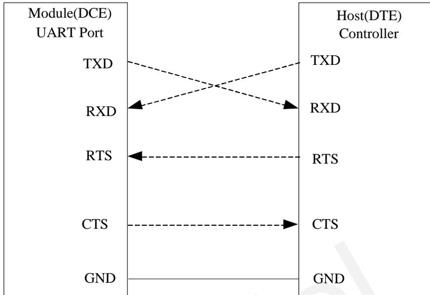
**Figure 20: Connection of UART port associated hardware flow control**
