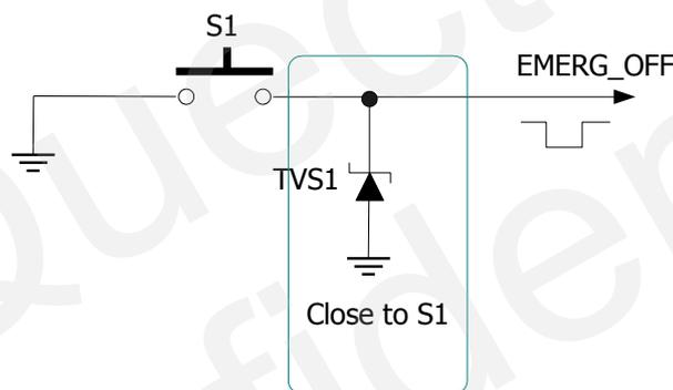
**Figure 11: Reference circuit for EMERG\_OFF by using button**
