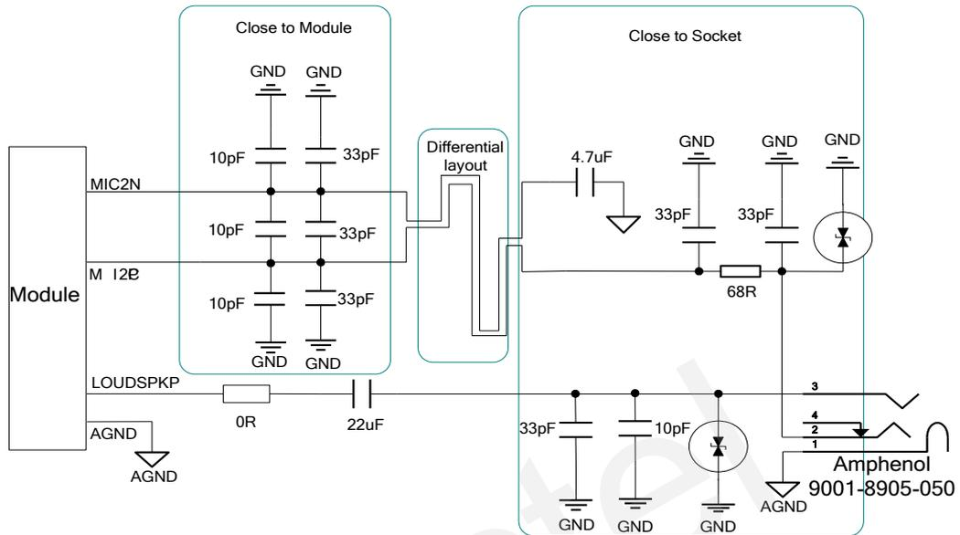
**Figure 28: Earphone interface design**
