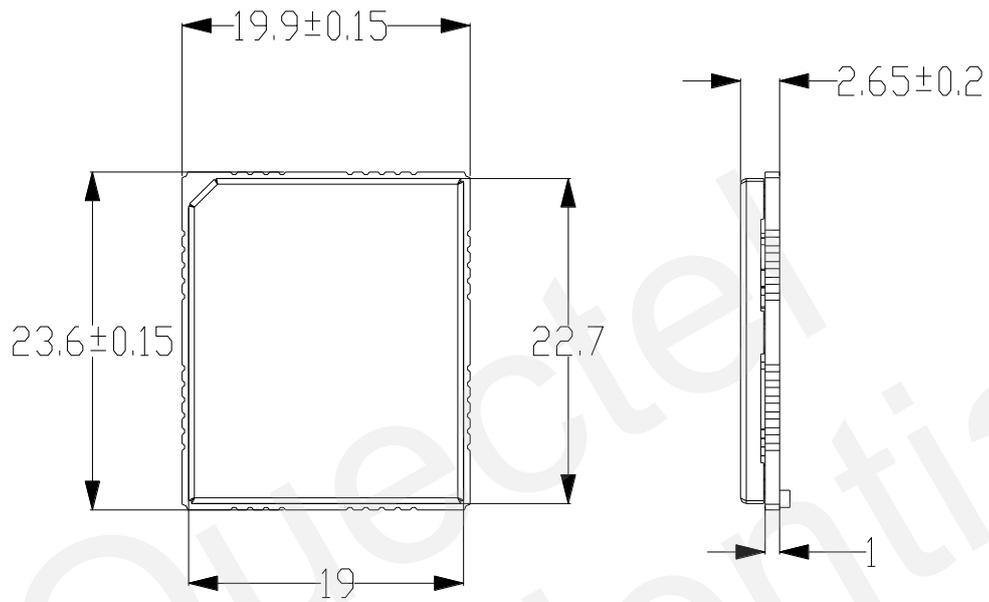
Figure 40: M35 top and side dimensions (Unit: mm)
