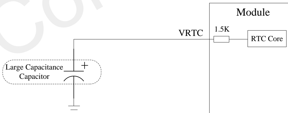
Figure 16: RTC supply from capacitor
