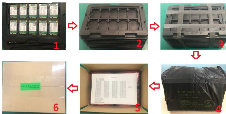
Figure 44: Tray Packaging Procedure
