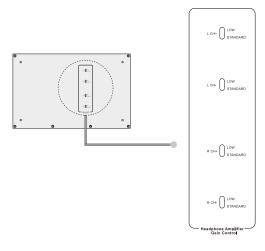
Headphone amplifier gain control switch: the default setting is "Standard" mode. When using in-ear monitors (IEMs), please set this to "Low" mode. Before use, ensure all four switches are set to the same setting.
