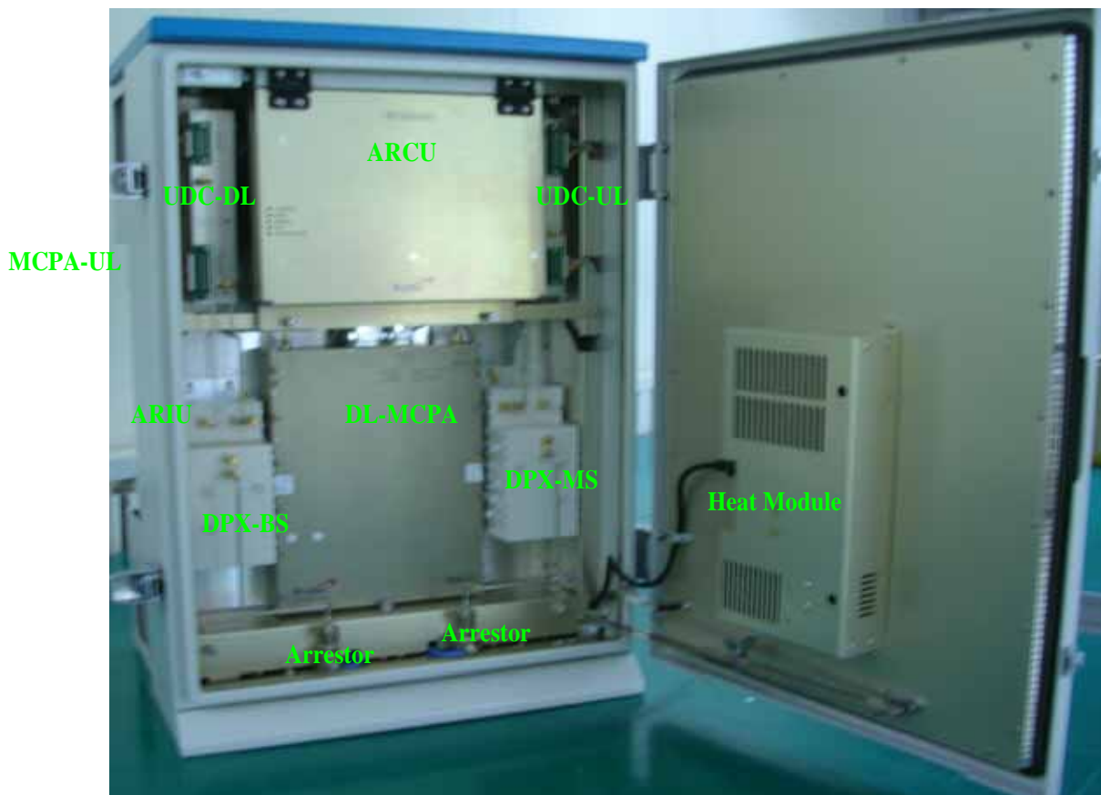
Figure 1 Sub units in a band selective repeater (Main Box)
