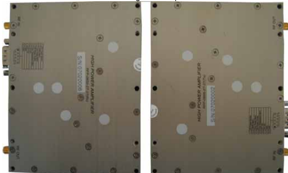
Figure 10. HPA(High Power Amplifier)
