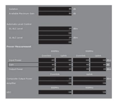
After running Easy Setup or Isolation Measurement, Isolation is displayed with "95" when the isolation is higher than 95dB, or it is displayed with the actual when the isolation is lower than 95dB.
