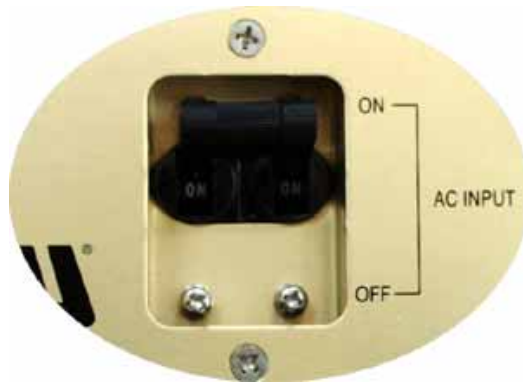
Figure 5.4 AC Power ON
