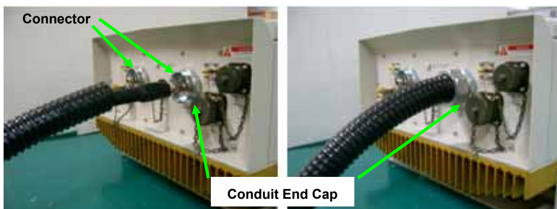
Figure 3.22 Installing the connector on the repeater side
