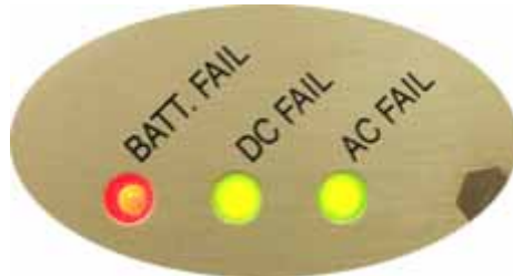
Figure 5.5 Power Alarm LED
