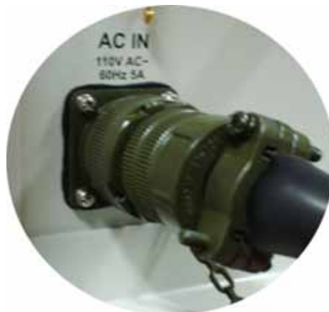
Figure 5.3 AC Power cable connection
