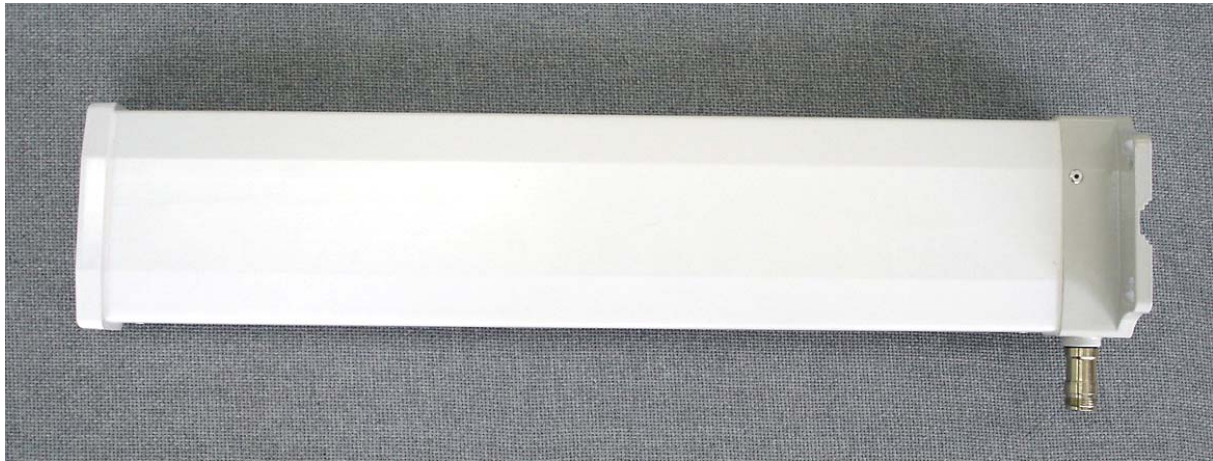
Figure 3.5 A Yagi antenna (Donor antenna)
