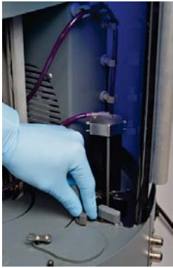
1. Free the rinsing tray by giving a quarter turn to the screw
