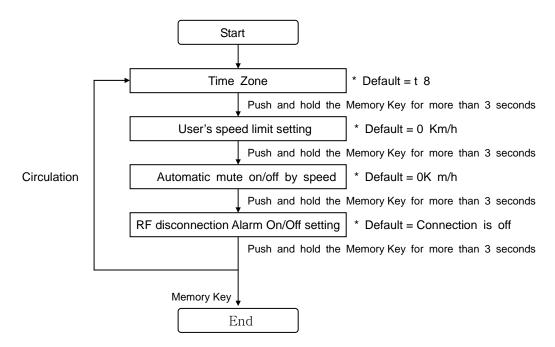
**MEM button:** When pushing the MEM button for 1 second, it will go to the next Time Zone. Holding for 6-7 seconds, the setting is finished and confirmed for the Time Zone selected.
