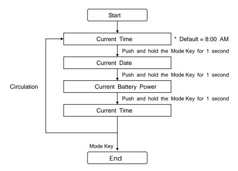
**MOD button:** When pushing the MOD button for 1 second, it will enter into the next mode. Holding for 6-7 seconds, the setting is finished and confirmed for the Mode status selected and return to standby.
