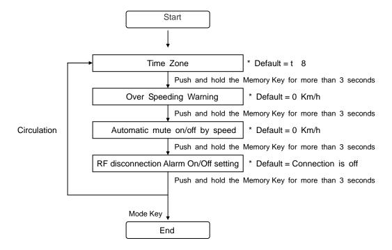
1-3 <u>Automatic Mute on/off by speed setting</u>: To avoid the signals from auto doors or micro towers when your speed is under limit selected in downtown, the "Mute"
