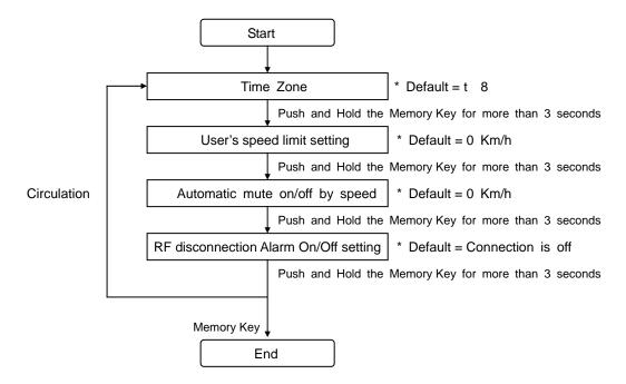
**MEM button:** When pushing the MEM button for 1 second, the function of RF disconnection Alarm will be off. Holding for 6-7 seconds, the setting is finished and confirmed for the status to be Off.
