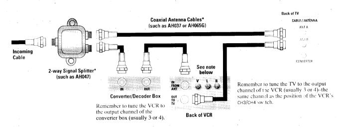
Most cable companies that require use of a converter/decoder box only require the box for scrambled premium channels like HBO or Showtime. All the other cable-TV channels can usually be viewed without the converter box. Therefore, by using a signal splitter, you can send the incoming cable-TV signals directly to the TV and also thru the converter/decoder box and VCR as shown above.
