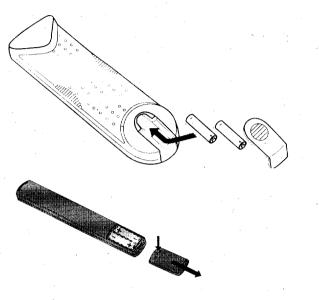
**3** Install the batteries in the compartment as shown.
