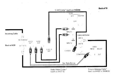
**Note:** Remember to also connect the video cable if you plan to use this VCR for picture-in-picture viewing or if you want to use the SELECT OUT jacks for recording. When recording from SELECT OUT jacks, tune the TV to channel 91 to see the signal from the S-VHS VCR.
