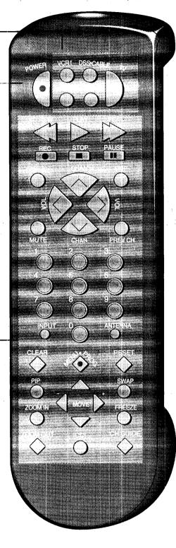
The ProScan universal remote that came packed with your TV also controls most brands of VCRs, cable-TV boxes, and selected RCA audio equipment.
