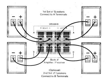
**Important:** When connecting the speaker wire, make sure you connect the (+) terminal on the amplifier or receiver to the (+) terminal on the speaker. One side of the speaker wire is usually marked with a white stripe to help you connect (+) to (+) and (-) to (-). If the (+) and (-) terminals are not matched properly, the speakers will not be "in phase" causing reduction in low frequencies (bass).
