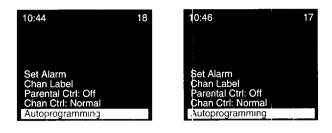
**5** When the TV finishes cycling, you can check which channels are in memory by pressir g the CHANNEL up or down button. Your set will stop on each of the channels in memory.
