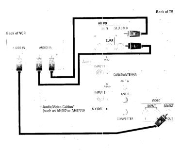
To see the signal from a device connected to the INPUT 1 jacks, select channel 91. Select channel 92 to see the signal from a device connected to the INPUT 2 jacks.
