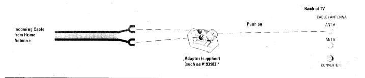
C. If your home antenna cable(s) are a 75-ohm, round, coaxial cable that carries VHF (channels 2-13) and a 300-ohm, flat, twinlead cable for UHF (channels 14-69), connect it to your set like this:
