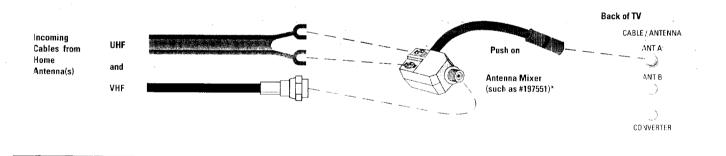
**D**. If the antenna cables coming from your home antenna(s) are two 300-ohm, flat, twin-lead cables as shown here, connect them to your set like this:
