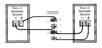
**Important:** When connecting the speaker wire, make sure you connect the (+) terminal on the TV to the (+) terminal on the speaker. One side of the speaker wire is usually marked with a white stripe to help you connect (+) to (+) and (-) to (-). If the (+) and (-) terminals are not matched properly, the speakers will not be "in phase" causing reduction in low frequencies (bass).
