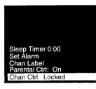
Repeat step 3 for each channel you want to lock out. If the PARENTAL CTRL function is set to ON while you are locking out channels, each channel will go blank as you lock it out.
