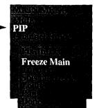
4 Repeatedly press the + or - button to highlight the Freeze Main function. Press the MENU button to freeze the picture. Press the MENU button again to return to normal video.
