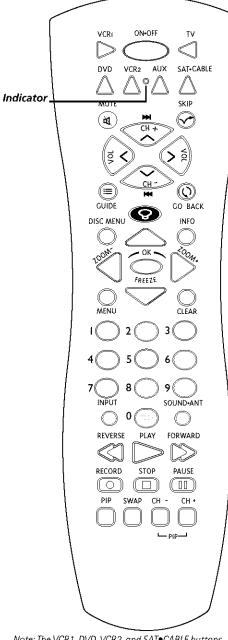
Note: The VCR1, DVD, VCR2, and SAT•CABLE buttons also turn on most RCA, GE, and Proscan products.
