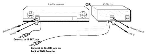
7. Place the wand in front of the remote sensor, approximately one inch away from the remote sensor.
