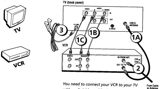
with audio/video cables in order for Picture-In-Picture (PIP) to work (see picture above).
