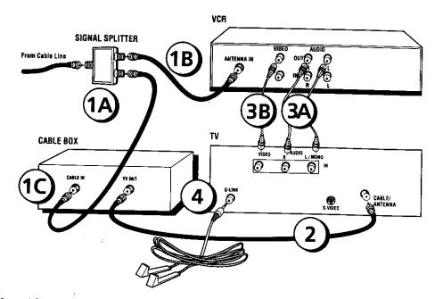
**Note:** The GUIDE Plus+ system's One-Touch VCR Recording feature is not available with this connection. If you want to use the One-Touch VCR Recording feature with your cable box, you must use the TV and VCR connection on page 8. You can do so by routing the signal from your cable box into the antenna input on your VCR. Note that PIP won't work if you use this connection. This connection may not be compatible with all cable services, especially if some or all cable channels are scrambled.
