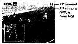
To change the PIP channel, press the channel buttons on the VCR. To change the TV channel, press CH CTRL until the TV channel is highlighted (yellow) and press the CH up and down buttons.
