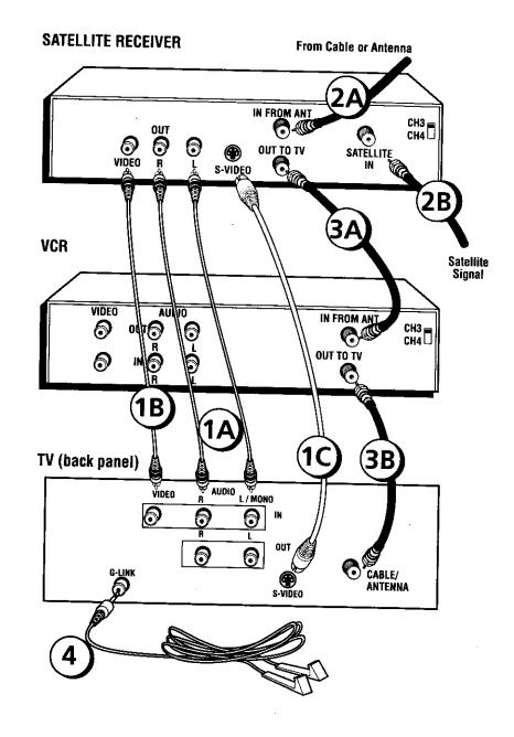
You need to connect your Satellite Receiver to your TV with audio/video cables (see picture above) in order for Picture-In-Picture (PIP) to work.
