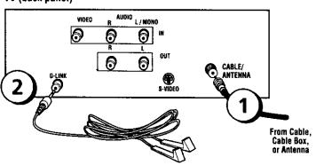
PIP (Picture-In-Picture) won't work if you use this connection. You must connect a VCR to your TV with audio/video cables in order for PIP to work.
