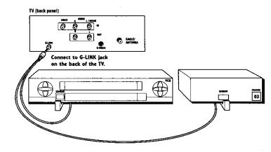
If you don't have both a cable box and a VCR connected to your TV, just coil the cable of the extra G-LINK wand with a twist tie and leave it behind the TV.
