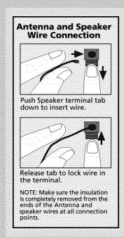
To ease speaker connections, the speaker cords and the terminals are color-coded.
