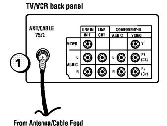
Note: This is the back of model T20TF668. If you have model T27TF668, you'll notice the ANT/CABLE jack is on the right side and it has a VIDEO LINE OUT jack.
