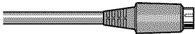
If your TV has an S-Video jack, connect an S-Video cable (optional). S-Video provides better video quality than composite video (the yellow jack).
