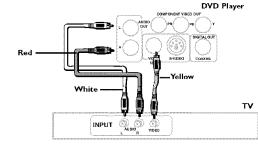
Note: Whenever you are connecting your system cables, turn off the power and make certain that the power cord has been removed from the wall outlet.
