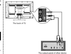
The picture below is an example of a connection using the HDMI video Digital Audio out: Connect a coaxial cable for digital audio output.
