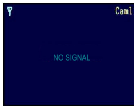
NO SIGNAL: The "NO SIGNAL" message means the receiver cannot access the camera. Please reposition the camera, or check the camera power.
