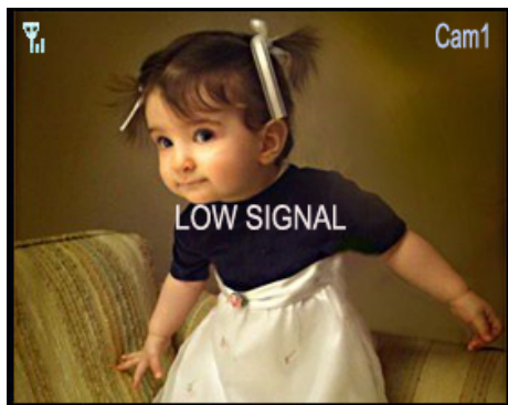
LOW SIGNAL: The " LOW SIGNAL" appears when the receiver has one or two bars. You will still get an image, however updating may be less frequent.
