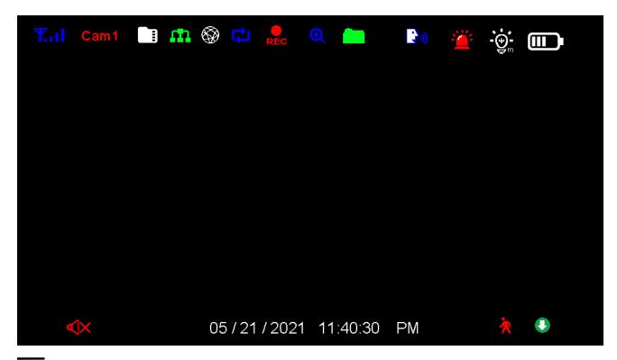
**Signal Strength:** Shows how strong the camera's signal is. Signal ranges from 4 bars down to 0 bars (out of range).
