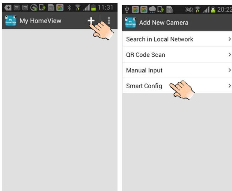
3) Input the local network password on the pop-up, then input camera password (000000) on next pop-up, touch "save" to complete the connection
