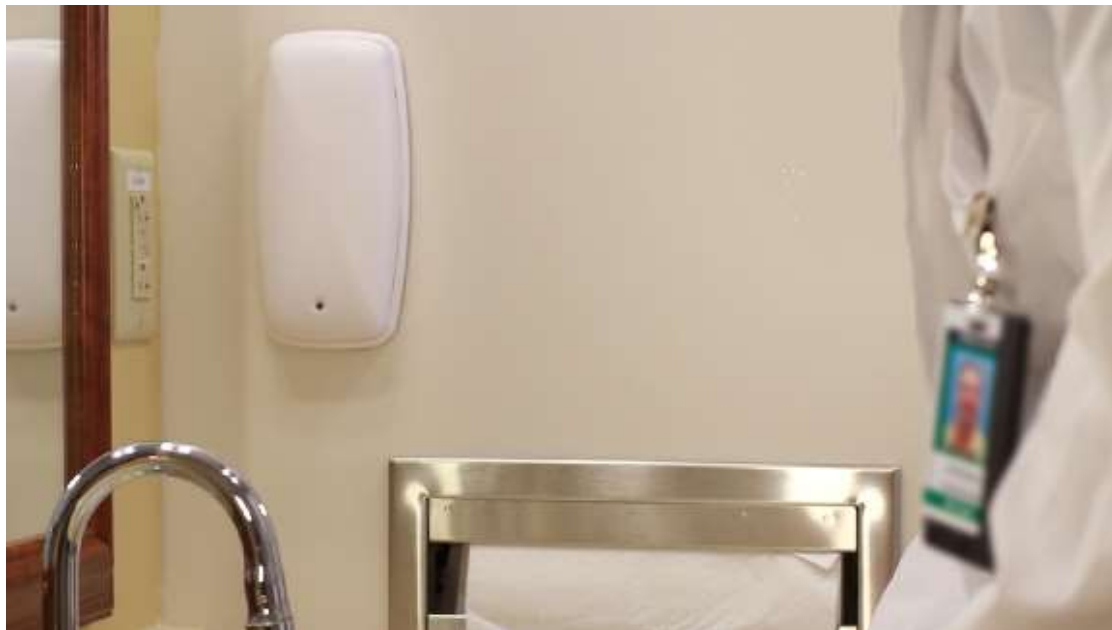
Figure: R142-I Badge Tag deployment with an A760 Proximity Locator to monitor entry and egress.
