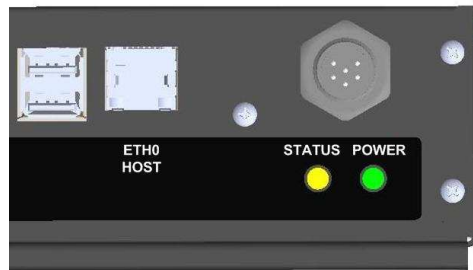
Figure 3 Array Controller Indicator Lights
