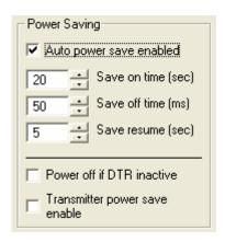
"Save On Time" sets the time that the transceiver is switched off for during the power save cycle (Power Save On). The Save On Time is programmable from 0 - 63.75 Seconds in 250ms (1/4 second) steps.
