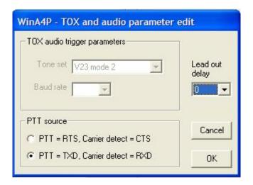
**"Ext TX on audio TOX"** routes the audio input via a Tone Operated Switch (TOX) which can be set to detect V23 or BELL202 formats in the "Edit | Modem/TOX/Protocol" menu. Detection of the selected format will key up the transmitter and forward the incoming data. To ensure that the radio does not key-up on noise, the TOX circuit checks for valid modem tones, not just the presence of some audio, before keying the radio.
