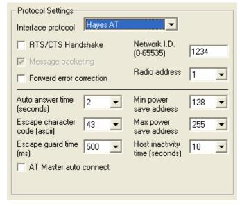
"Escape Character Code" field is only available for Hayes AT protocol and allows the user to define the desired escape code.
