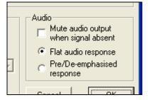
By placing a tick in the "Mute Audio" check-box, the receive audio path can be set to mute when no incoming carrier is detected. If this option is not selected, background noise could cause connected modems to generate spurious characters at extremely low RF signal levels.
