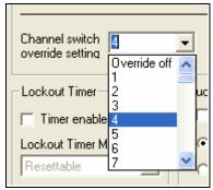
The CRX receivers do not have any front panel switches for channel selection. On that product, you can still program a number of frequencies into the different channel numbers in the same way, but the "Channel Switch Override" becomes the primary method of selecting the desired operating channel. The labelling changes to "Rx Channel" to reflect this.
