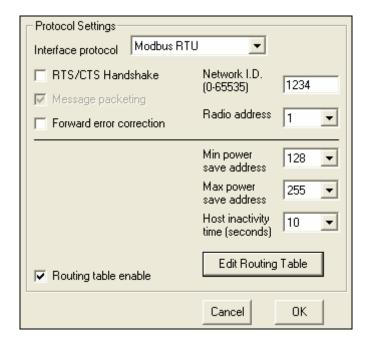
"Min Power Save Address" & "Max Power Save Address" define the limits of the range of radio addresses for which power save mode will be active when Modbus or RFT Routing Protocols are selected. Radios with addresses outside this range will not use power-save.
