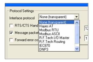
In these protocol specific modes, the radio recognises a complete message frame and only transmits data which conforms to the specified format. These modes also allow routing modes to be enabled in which messages can be passed down a chain of radios using "Store & Forward" techniques.
