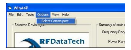
A small sub-window will appear with a pull-down menu allowing selection of port Com 1 to Com 16. Once the required port is selected, press OK to proceed. On most PCs with a single serial port, this port will be Com1.
