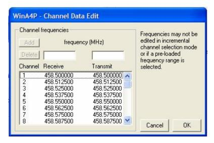
In discrete mode, the program will allow you to edit the data in the frequency table. To add a new channel, highlight the position in the table where you would like to add the new channel, type the required TX and RX frequencies in the small entry fields, then click on the "Add" button. To delete a channel, simply highlight the relevant row in the table, then click on the delete button (or press "Delete" on the keyboard).
