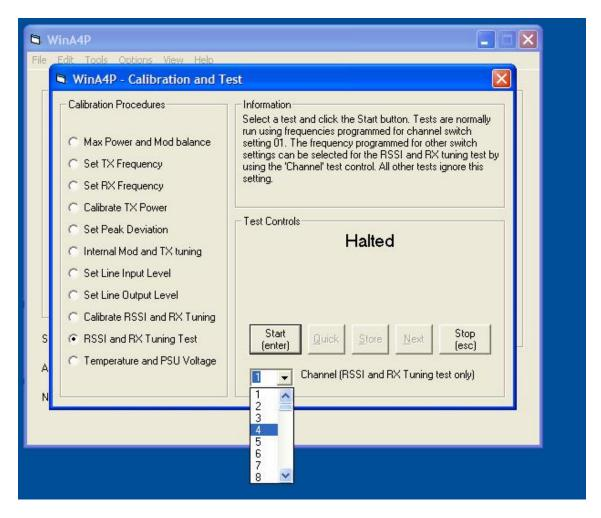
When you click the Start button on screen (or press the Enter key), the receive signal level will be shown as a bar-graph with a digital readout above it.
