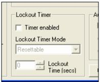
"Lockout Timer Mode" allows either resettable or cumulative mode to be selected. In resettable mode, transmission will cease after the programmed time and will not restart until the action that normally causes transmission is removed then re-applied. The timer resets and starts counting up again each time a transmission starts.
