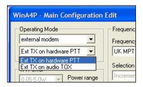
**"Ext TX on Hardware PTT"** sets the radio to key up when a "Push to Talk" signal is applied to the appropriate input pin. The PTT input connection arrangement differs between the various radio models which can accept external audio, but full details are given in the individual radio manuals. In particular, the URT Series has a two different options available with regard to which pins on the 25-way connector are used for PTT. These can be selected from the "Edit | Modem/TOX/Protocol" menu.
