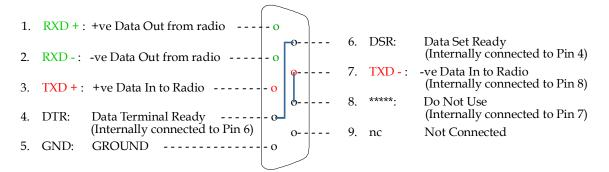
When half-duplex (2-wire) RS422/RS485 operation is programmed, the TXD- and TXD+ signals are internally connected to the RXD- and RXD+ signals respectively. The 2-wire half-duplex bus only needs to be connected to the RXD- and RXD+ pins (Pins 1 and 2). Shorting links are not required in the connector.
