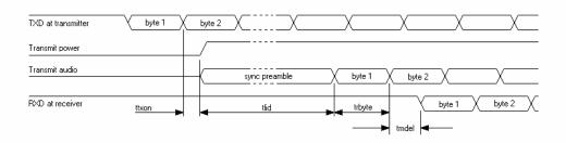
The time delay between receipt of the stop bit for the first character to be transmitted at the transmitting radio and output of the start bit of that character at the receiving radio is the sum of the values ttxon, tlid, trbyte, and tmdel shown in the diagram above. Values for these parameters are indicated below:
