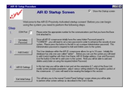
**Step 1 -** Enter the COM Port on which the AIR ID base unit is attached. This function will test the communication with the base unit. If the AIR ID software cannot communicate with the base unit, an error message will be displayed. If an error occurs, check that the Base Unit is properly attached to the system and the correct port number is being used.
