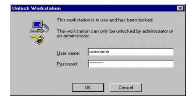
Once the cursor is in the Password field, the user may safely wave their proximity token over the pcProx reader and the field is stuffed with the password. The user may finish off the operation by pressing the ENTER key, or the reader may be configured to add the ENTER keystroke as an appended keystroke.
