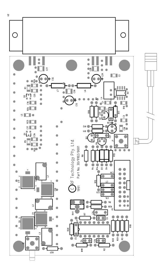
Figure 7: The component overlay diagram for the lower-power PA board
