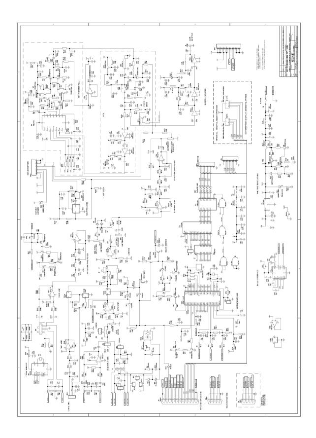
Figure 3: The component circuit diagram of the 9103 UHF Transmitter.
