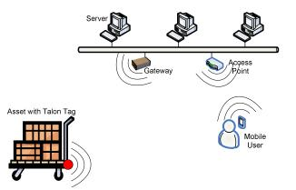
Once this communication is complete the Talon tag goes to a stationary power saving state and begins transmitting its heartbeat if turned on.
