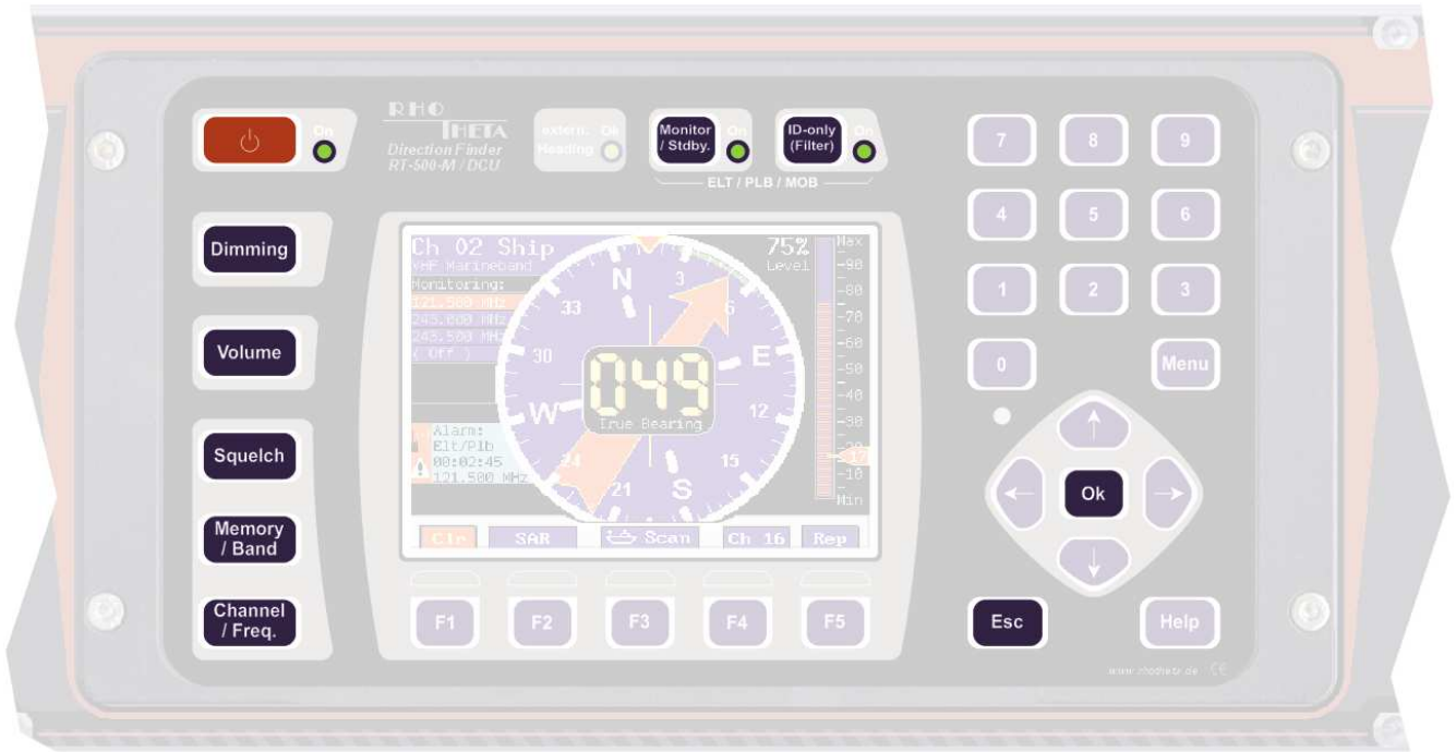
Fig. 20 Operating and adjusting
